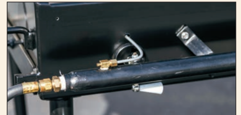
Gas Manifold With Cover Removed
