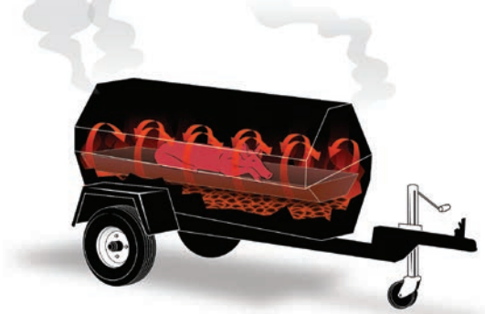
The removable drip pan between the fire and the food creates vertically indirect heat.
