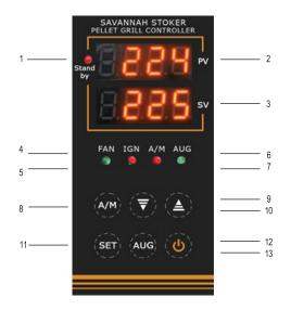
(1) Stand by indicator: Light is on when the controller is connected to a power source but not running. When the controller is running the light will go off and the displays will be on.
